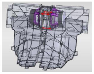
This audio system is completed by two woofers for the 80 Hertz to 20 Hertz frequency range. They are hidden inconspicuously between the seats.
