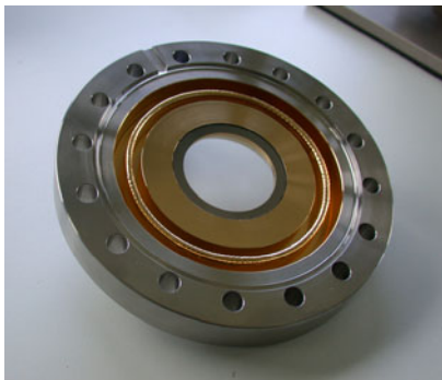
CVD diamond window in UHV flange
