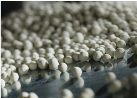
Zeolite balls help to reduce power consumption in dishwashers of BSH Bosch und Siemens Hausgeräte by up to 30 percent.
