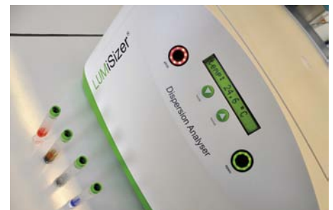
LUMiSizer ® for analysis of suspensions (stability, particle size distribution).
